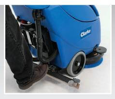
**Foot-activated squeegee** Foot-activated squeegee lift enables operators to easily maneuver the machine.
