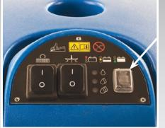
**Easy to use control panel** Electronic solution control for low, medium and high flow.
