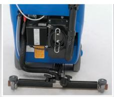
**Center-pivot squeegee system** Center-pivot squeegee system employs a gas spring for maximum blade pressure to ensure complete dirty solution pickup in both forward and reverse.
